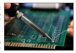
be extremely hot during and after soldering work, and they can easily burn the skin through contact. Moreover, they can also cause a fire if placed on flammable or combustible materials.
