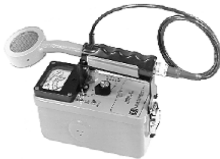
GM on a Survey Meter
