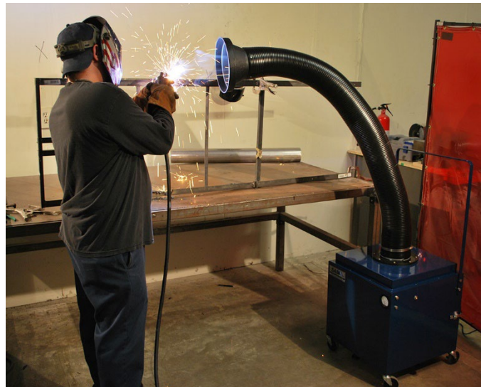
Figure 5. Example of a portable fume extractor that can be manipulated and moved depending on the operator needs.
