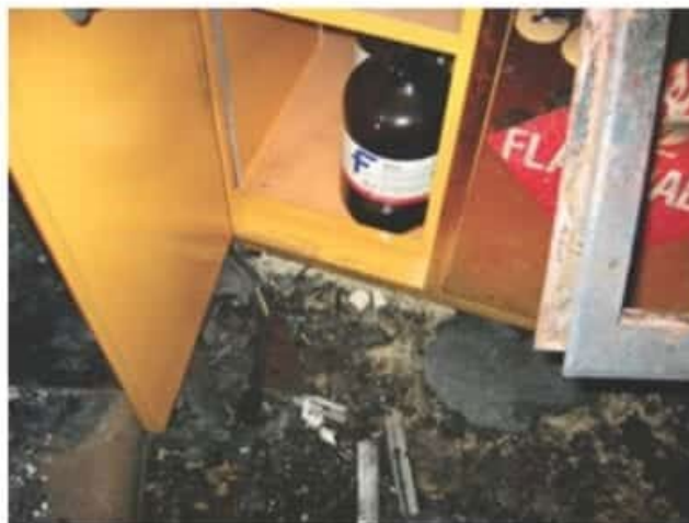
Figure 2: Flammable chemical unaffected by the fire outside of a flammable storage cabinet.
