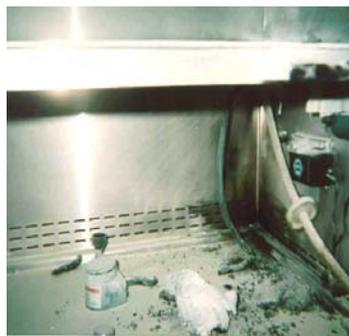
4.9.1 Use of gas in BSC's has led to fires, compromised HEPA filters, destroyed cabinets and injured workers.
