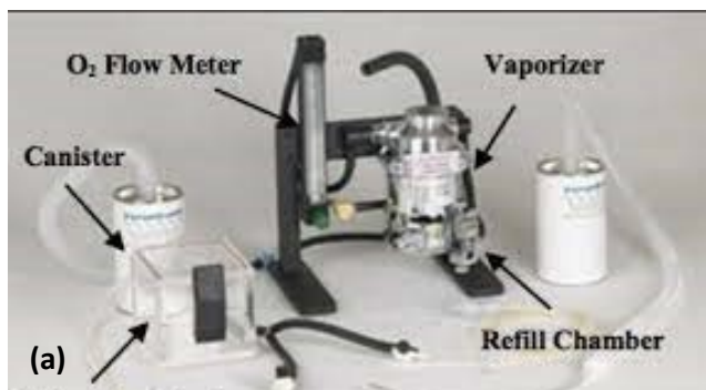
Fig. 1. (a) Example of passive scavenging system. (b) Charcoal filtration system.
