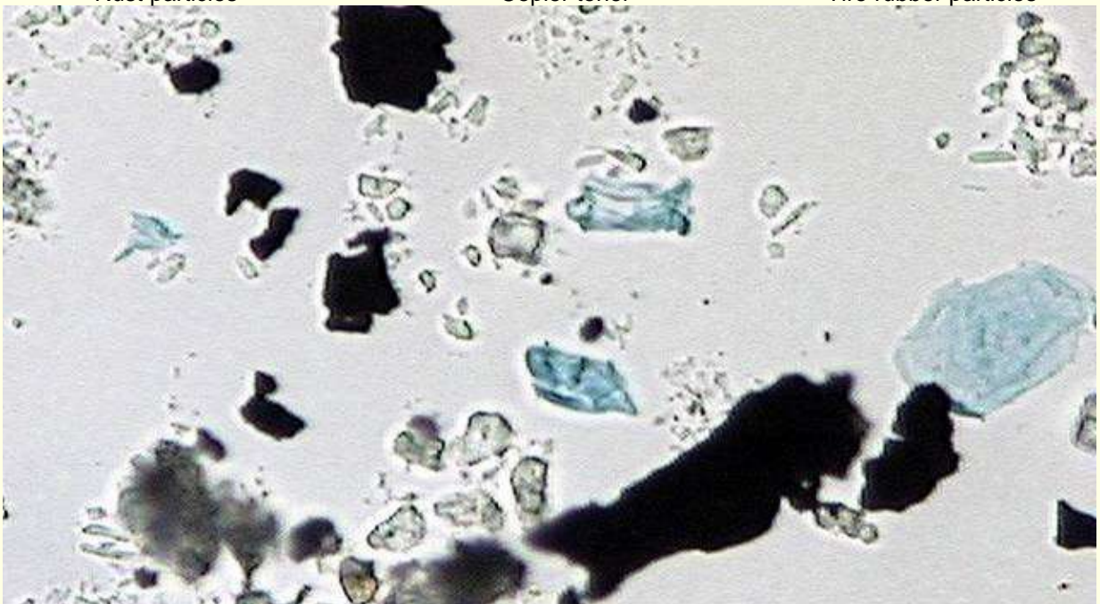
Example of "high" opaque particle loading from HVAC system shedding
