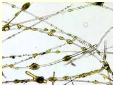
Yellow duct wrap insulation
