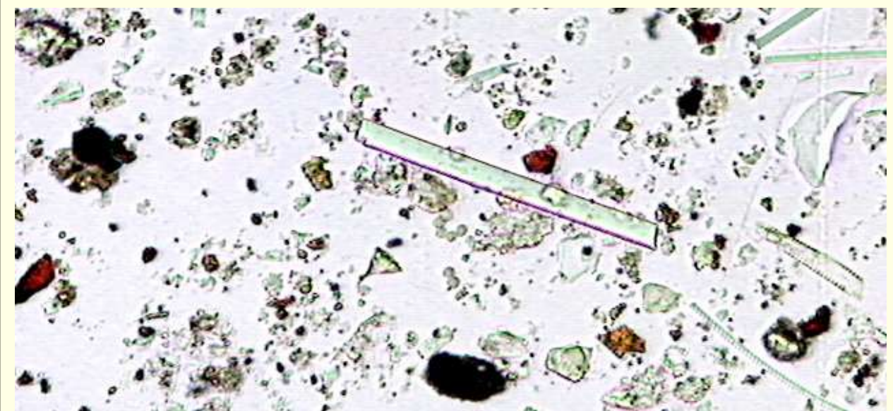
Mixture of rust & opaque particles (and mold spores) in construction debris – 800X
